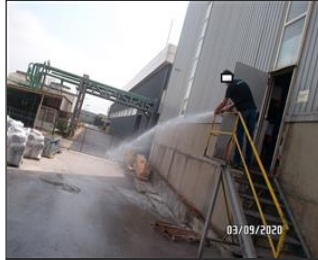
Photo of fire safety equipment Fire hose tested-2.JPG
