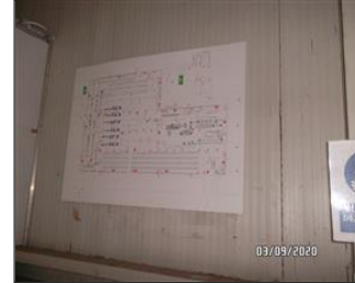
Photo of fire safety equipment NC7.16-CORRECTED-Evacuation plans are posted on walls next to the exit doors in the production area.JPG
